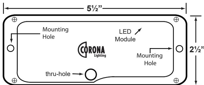
**NOTE:** This is the back of the Fixture. Looking from the front of the fixture the positions of through-hole and other details are reversed.
